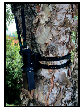
BRACKET with latching straps on a tree attached to the PLATE
